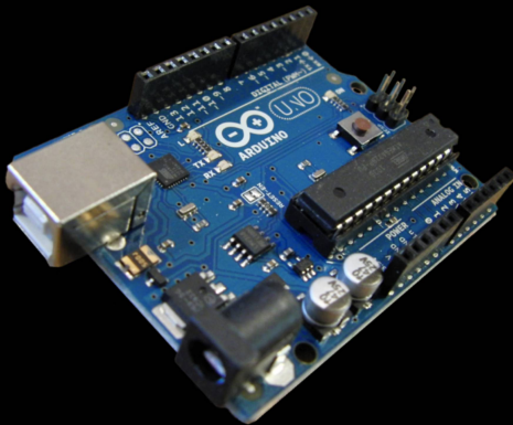
Arduino Uno board 8-bit Atmel AVR
